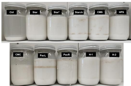
Figure 2. Appearance of 4-component fluids after hot rolling for 16 h.
