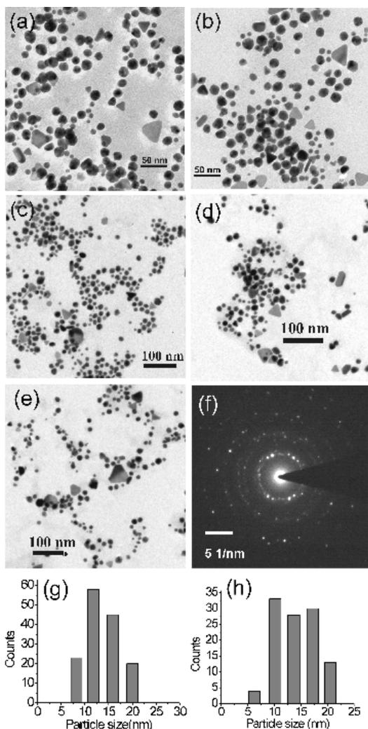
Figure 2: HRTEM images of stabilized AuNPs at various concentration of the fruit extract: (a,b,c) concentration =  $800 \text{ mgL}^{-1}$ ; (d,e) concentration =  $1000 \text{ mgL}^{-1}$ ; (f) SAED image of AuNPs and (g,h) histograms showing particle size distribution at  $800$  and  $1000 \text{ mgL}^{-1}$  concentration of the fruit extract.
